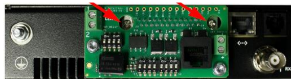
Rear of TB7300 with isolation adapter fitted
