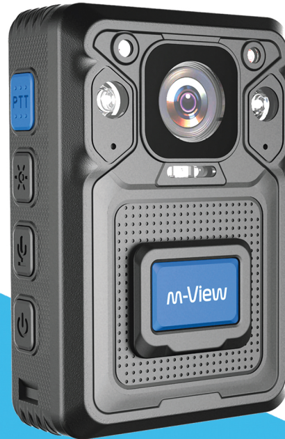
Dimensions - 84.5 * 56.3 * 27.3mm Weight - 162g (without mount)
